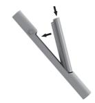
Now push the top part of the battery into the frame, until you hear the battery lock into position.
