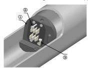
Insert the lock with the matching key into the round hole on the side of frame. Then insert the upper support into the frame and make sure the top of lock cylinder passes through the round hole on the upper support. Use one ST2.6\*16 screw and three M3\*10 screws to tighten the lock and upper support.
